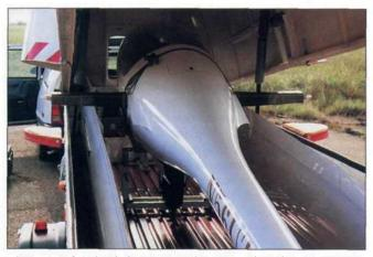
The SZD-56-1 loaded in its trailer. Note that the wing carrythru spar, which is permanently attached to the fuselage, extends about 18 inches beyond the fuselage sides. Therefore, to keep the trailer from being overly wide, the fuselage is stowed somewhat elevated on its support dolly with the fuselage spar above the zving trailing edges.
