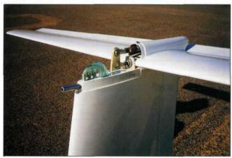
The horizontal tailplane locked onto the top of the vertical fin before the fairing is installed. The elevator control link is manually connected to the vertical control arm.
