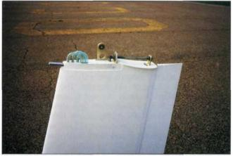
The top of the vertical tail fin before the horizontal tail is installed. The stabilizer attachment pin and lugs are to the right, and the elevator control arm is protruding upward in the middle.
