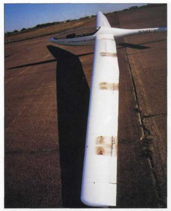
The SZD-56-1 wing after a 60 kt oil flow test flight. The oil patterns indicate that low drag laminar flow was achieved on the wing top surface aft to about .56 of the chord fraction, followed by normal attached turbulent flow to the wing trailing edge. The thinned oil flow chordwise streaks shown near the center of each oil test pattern are intentionally created turbulent wedges caused by the .008 inch high black tape "bugs" attached to the wing surfaces ahead of the oil test areas.
