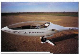
The fuselage on its support stand ready to accept its wing panels.
