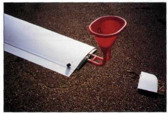
An innovative fiberglass funnel is plugged into the wing tips to load water ballast into the separate forward and aft wing tanks. Note the rubber stopper, shown near the wing trailing edge, that is used to plug one of the funnel's outlets when only one tank needs to be filled. The temporarily removed wing tip shown on the ground to the right.
