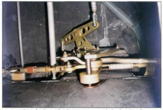
A view thru the large fuselage top access hole showing the manually connected flapperon links at the left and right hand sides. Note the all-carbon fuselage construction.
